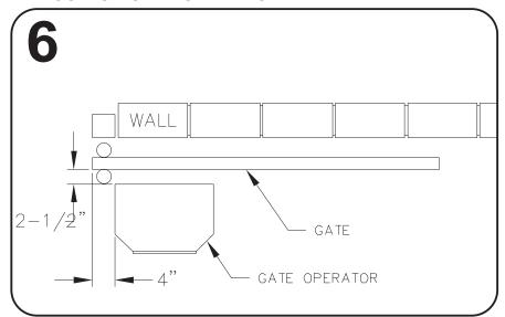
O If the steel mounting stand was used, simply bolt the gate operator to the stand. If the operator will be mounted to a concrete surface or pad, place the shortest edge of the operator 4" away from the edge of the driveway. Place the longer edge of the gate operator 2-1/2" away from the gate.
